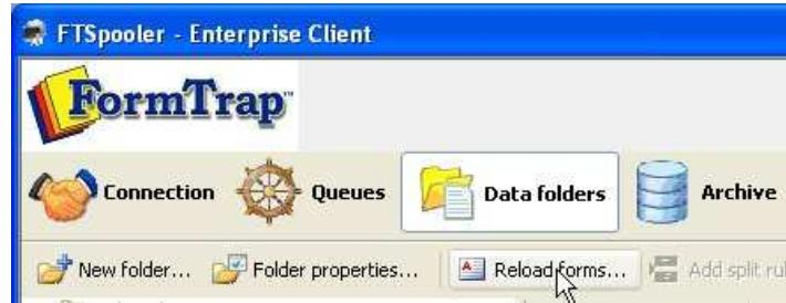
Version 7.1 can use 6.4 files without any subsequent Build or Reload forms. Earlier version files cause an error message from **formtrap.exe**.
